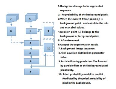
Figure 1 : Algorithm overall flow chart
