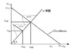
**Figure 1: Equal life curve and stress- strength interference relationship**
