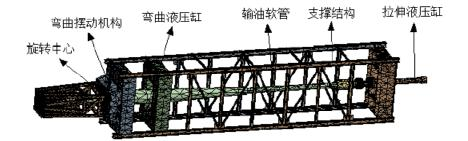
Figure 2: Structure model of fatigue testing machine
