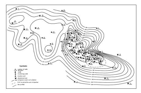
Fig. 1: Contour map of "Akirtobe" UGS confining reservoir bed
