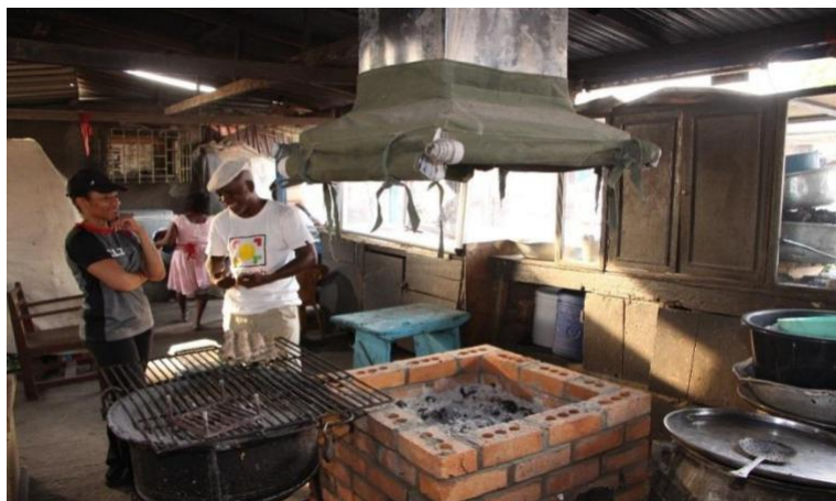
FIG. 6. Charcoal fish smoking cook-stove as an approach to replace the old stove made from a car rim closer to it
