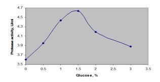
FIG. 5: Effect of glucose concentration on acid protease production.
