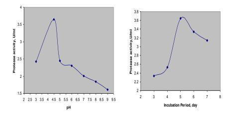
FIG. 1. Effect of pH and incubation period.(a) pH of fermentation(b) Time of incubation
