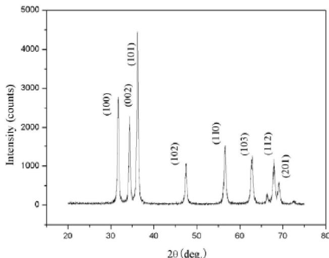
Figure 1 : XRD pattern of ZnO nanorods
