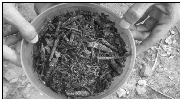
Fig. 1: Biochar obtained after drum pyrolysis
