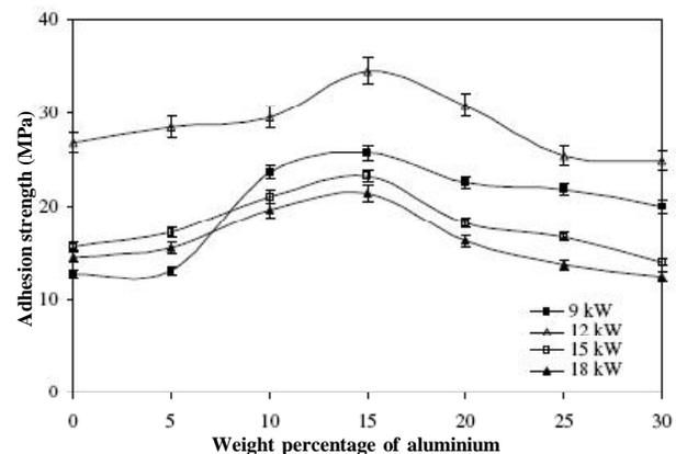
**Figure 3 : Variation in coating adhesion strength with aluminum content in the feed stock**
