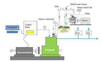
Fig. 3.1 Experimental setup
