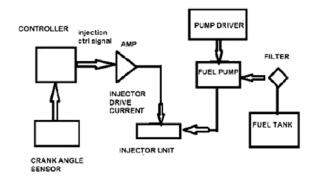
Fig. 4.1: Block diagram of Electronic Fuel Injection (EFI) system
