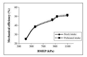
Fig. 5: Variation of mechanical efficiency with respect to BMEP
