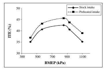
Fig. 7: Variation of ITE with respect to BMEP
