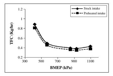
Fig. 4: Variation of TFC with respect to BMEP
