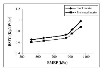
Fig. 3: Variation of BSFC with respect to BMEP
