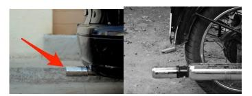
FIG. 2. Device used to collect vehicle emission.
