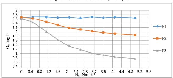
FIG. 5. Change of oxygen concentration in the wine at flow rate 26,3 m<sup>3</sup>.h<sup>-1</sup> with the growing flowrate of the injected nitrogen. Measured in the visors P1,P2 and p3.
