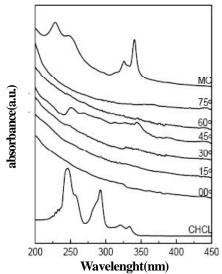
Figure 1: UV-Vis absorption spectra of mixed LB films of CA(0.5M) in SA matrix placed at angles 0°C, 15°C, 30°C, 45°C, 60°C and 75°C with the incident radiation alongwith the CA solution and microcrystal spectrum
