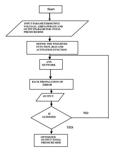
Fig. 3: Flow chart for neuron model of fan
