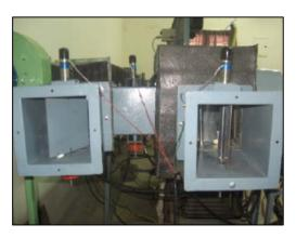
Fig. 7: View of supply and return duct system
