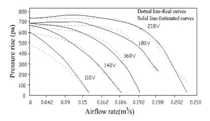
Fig. 8: Estimated fan performance curves for polynomial model
