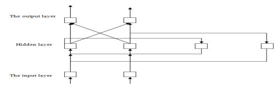
Figure 3 : Elman neural network model MODEL COMBINATIONS
