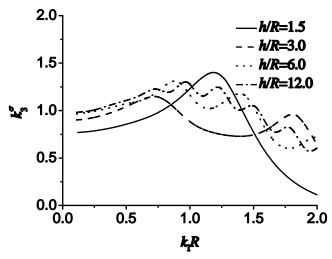
Figure 10 : Variation of DSIF vs. wave number and h/R
