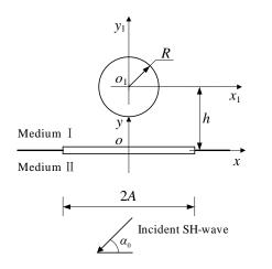
Figure 1 : Interacting interface crack and a circular cavity in a piezoelectric bimaterials
