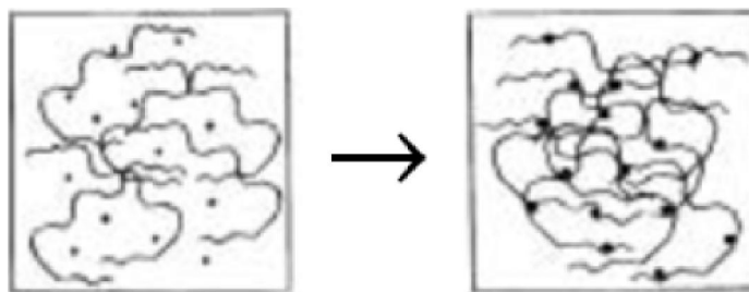
Preliminary scheme of microencapsulation of ions of metals by polymers [1]
