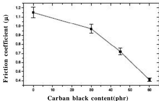
**Figure 1 : Course of friction coefficients as a function of CB content**
