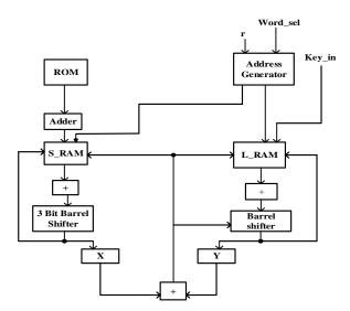
Fig. 1: Key expansion architecture
