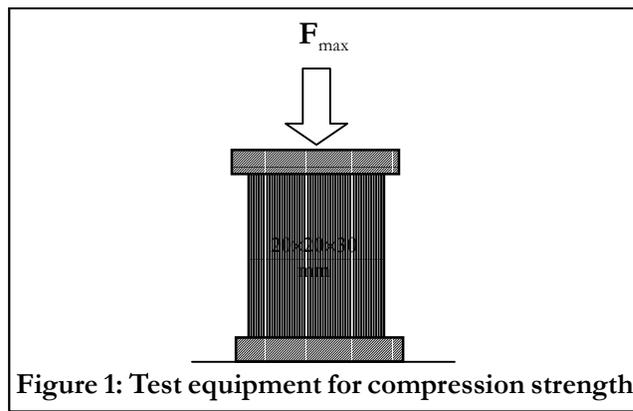
Figure 1: Test equipment for compression strength
