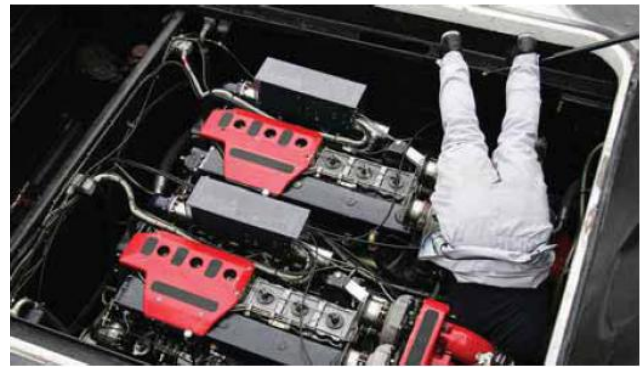
Figure 24 : Poor access to engine tools
