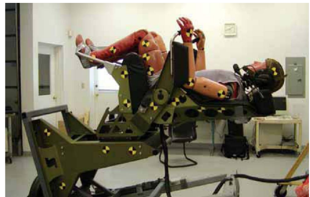
Figure 27 : Laboratory based anthropometric crash test on suspension test [15]
