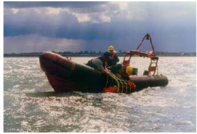
Figure 16 : An example equipment- That is designed for the recovery of man-overboard victims [19]
