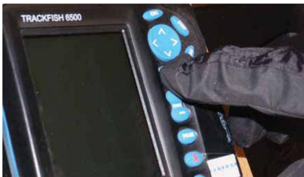
Figure 18 : Example of the difficulty operating SFB displays when using gloves [15]
