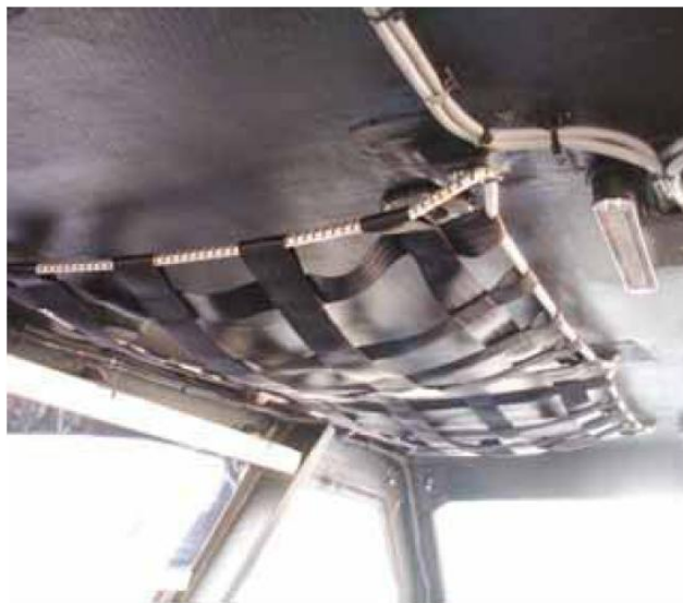
Figure 23 : Example of roof storage method on a SFB [15]
