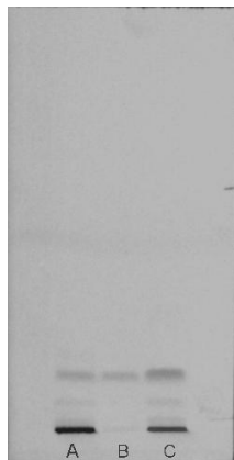
Figure 2 : TLC plate showing separation of eugenol in; (A) Methanolic extract of leaf powder of Pimenta dioica (L.) Merrill; (B) Standard eugenol and; (C) Methanolic extract of berry powder of Pimenta dioica (L.) Merrill
