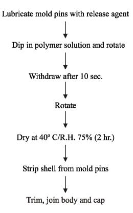
Fig. 2: Manufacture of asymmetric membrane capsules by dry process method
