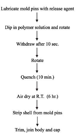
Fig. 1: Manufacture of asymmetric membrane capsules by wet process method
