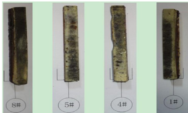
Figure 3 : The adhesion conditions of honing oilstone.
