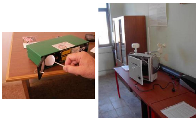
Figure 2 : Environmental dust monitor, GRIMMEDM 107.
