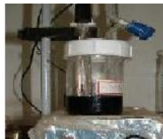
Figure 1: A two-in-one cell set up for potentiometric analysis with magnetic bead stirrer
