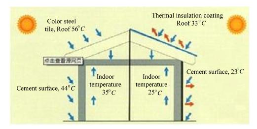
Figure 3: Effect of heat insulation for building energy-saving diagram
