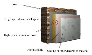
Figure 1 : Figure of building structure energy-saving implementation
