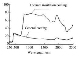
Figure 4: coating reflection spectra
