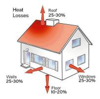
Figure 2: The diagram of the Maintenance of structural heat radiation
