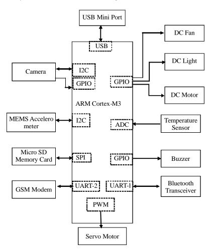
Fig. 1: Block diagram of E-Gateway
