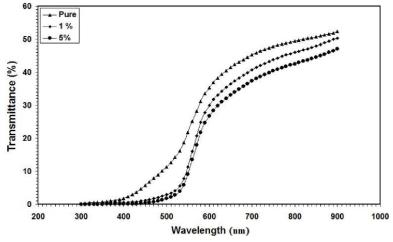
Figure 1 : Transmittance versus wavelength for pure and Co-doped CdO films
