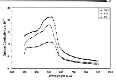
Figure 3 : Optical conductivity versus wavelength for pure and Co-doped CdO films
