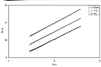
Figure 5: The lná versus hõ for pure and Co-doped CdO films TABLE 1 : The optical parameters
