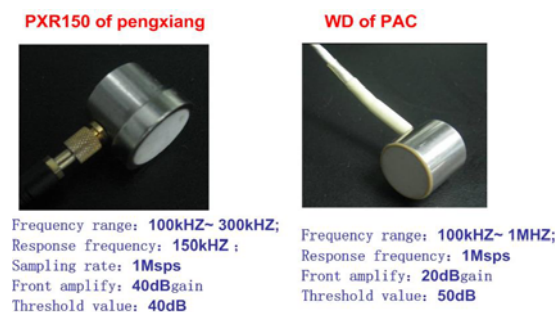
Figure 1 : Two types of sensors and their parameters
