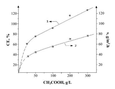
Fig. 2: Effect of concentration of acetic acid on current efficiency (1) and the dissolution rate of the metal (2) (i = 50 A/m<sup>2</sup>;  $\tau$  = 0,5 h.; t = 25°C)
