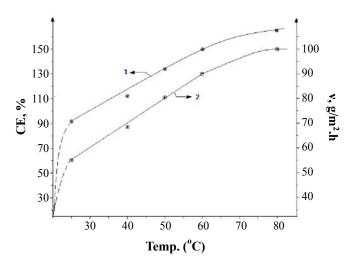
Fig. 4: Effect of temperature on the current efficiency (1) and the dissolution rate of zinc (2) (C<sub>CH3COOH</sub> = 100 g/L; i <sub>Zn</sub> = 50 A/m<sup>2</sup>; τ = 0,5 h)
