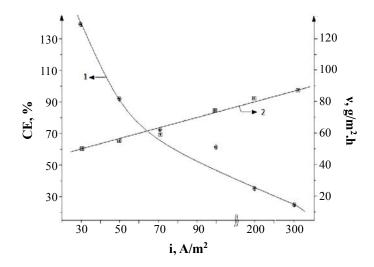
Fig. 1: Effect of current density of the zinc electrode on current efficiency (1) and the dissolution rate of the metal (2) (CH<sub>3</sub>COOH = 100 g/L,  $\tau$  = 0,5 h, t = 20°C)
