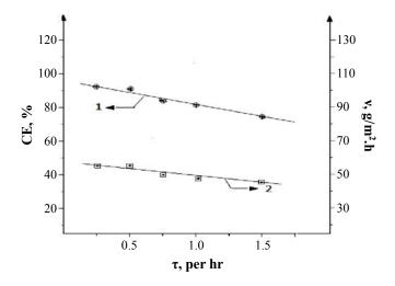
Fig. 3: Effect of the duration of the electrolysis on current efficiency (1) and the dissolution rate of zinc (2) (CH<sub>3</sub>COOH = 100 g/L; i = 50 A/m<sup>2</sup>; t = 25°C)
