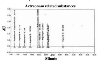
Figure 4: Chromatogram of Aztreonam sample spiked with its impurities in 1% level
