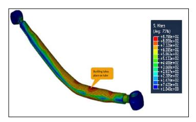
Fig. 5: Displacement plot for Ø50 x 6 tube buckling load: 10150 kg
