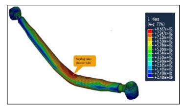
Fig. 4: Displacement plot for Ø50 x 6 tube buckling load: 9276 kg
