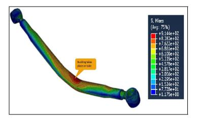
Fig. 2: Displacement plot for Ø50 x 6 tube buckling load: 7650 kg
