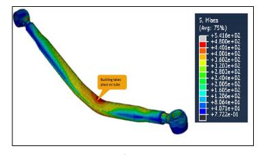
Fig. 1: Displacement plot for Ø50 x 6 tube buckling load: 4054 kg
