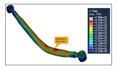
Fig. 3: Displacement plot for Ø50 x 6 tube buckling load: 5445 kg
