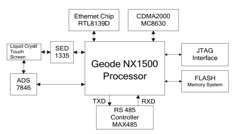
Figure 2 : Embedded-based system of intelligent home hardware platform structure
