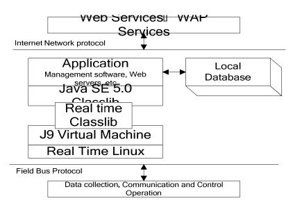
Figure 3 : The structure diagram of intelligent home gateway
