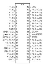
Figure 1: AT89C51 microcontroller pin chart
