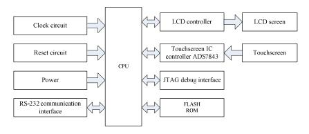
Figure 3: Hardware design framework
