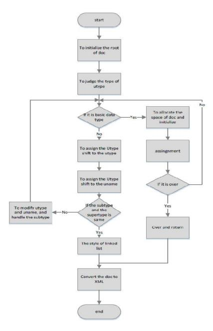
Figure 6: Mechanism of encoding process
