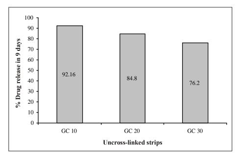
Fig. 1: Comparative release profile of polymeric strips containing gatifloxacin for uncross-linked strips<sup>\*</sup>
