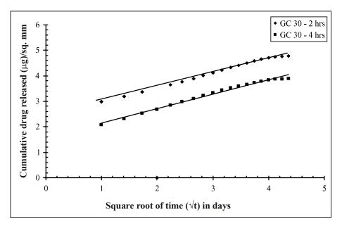
Fig. 6: Best fit lines for Higuchi's equation for cross-linked chitosan strips containing gatifloxacin
