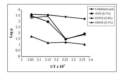
Fig. 2: Plot of corrosion rate Vs temperature
