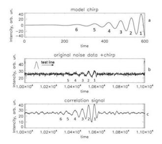
FIG. 2. Scheme of proposed correlation method.
