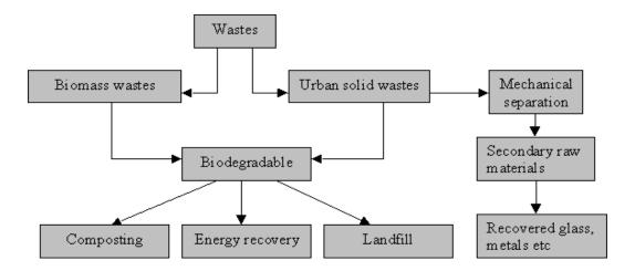
FIG. 3. Mapping for the treatment of solid waste for the process of recovery and recycling.
