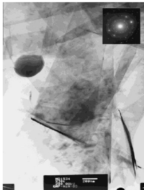
Figure 3 : TEM micrographs of GNP in transmission regime and selected area electron diffraction regime (in the right angle)
