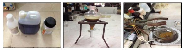
Fig. 1: Raw jatropha oil, methanol & catalyst, separating funnel, flask cum stirrer & external heater
