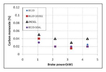
Fig. 6: Variation of carbon monoxides with load
