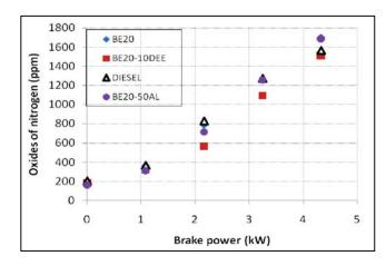
Fig. 5: Variations of oxides of nitrogen with load
