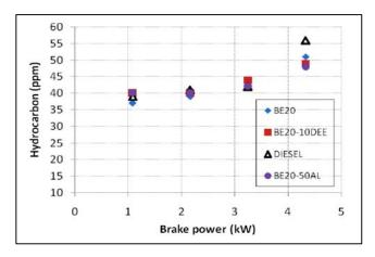
Fig. 7: Variation of unburned hydrocarbons with load
