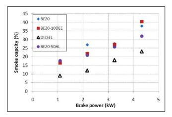
Fig. 8: Variation of smoke opacity with load
