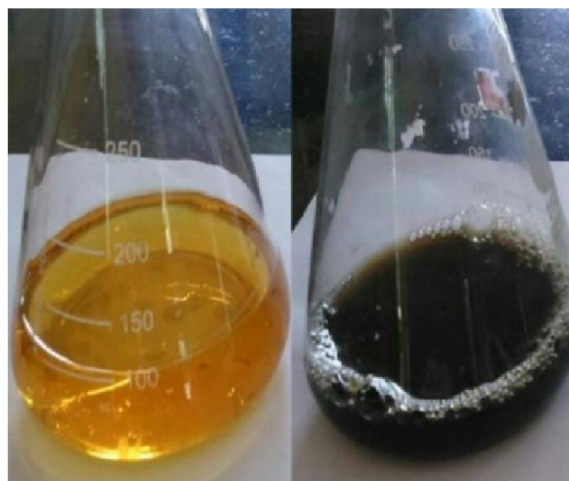
Figure 1 : Color change from yellow to black on synthesis of iron nanoparticles
