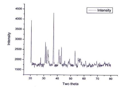
FIG. 4. XRD pattern of Ni nanoparticles obtained from coriander leaf extract.
