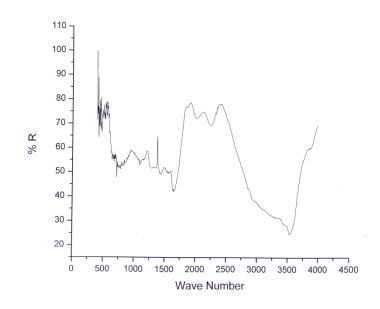
FIG. 3. FTIR spectrum of synthesized of Ni nanoparticles using coriander leaf extract.
