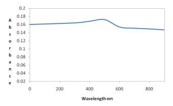
FIG. 2. UV-Vis spectrum of nickel nanoparticles dispersed in deionized water at room temperature.
