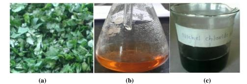
FIG. 1. Steps for synthesis of nickel nanoaprticle. a) Coriander leaves; b) Coriander leaves extract; c) Nickel chloride solution 0.1 M, coriander leaves extract, and nickel nanoparticles settled at bottom.
