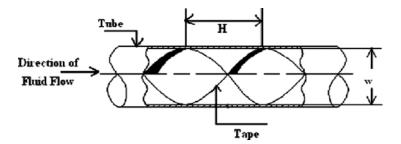
Fig. 2: Twisted tape model
