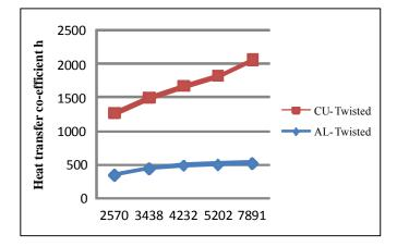
Fig. 5: Shows the variation of Reynolds number and heat transfer co-efficient
