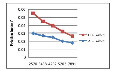
Fig. 6: Comparison of Reynolds number and friction factor
