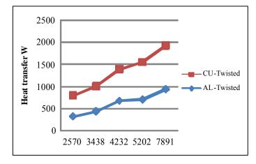
Fig. 3: Comparison of Reynolds no and heat transfer
