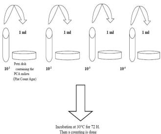
Sampling technic on the tested surface of the unit
