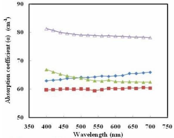
Figure 5 : The absorption coefficient ( $\alpha$ ) of bone/matrices pre- and post-demineralization using different acids as a function of wavelength
