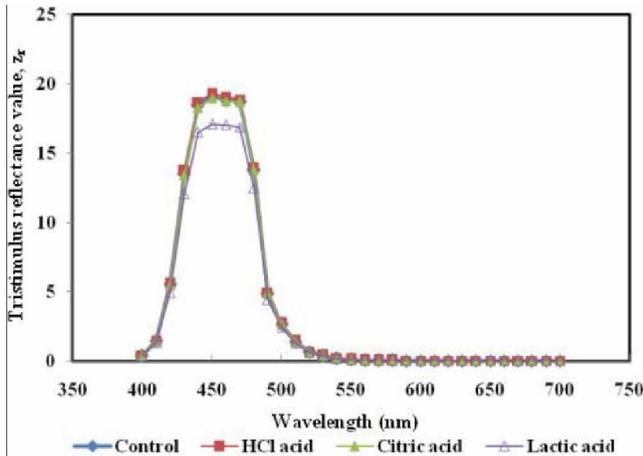
Figure 4 : Variation of the tristimulus reflectance value ( $z_r$ ) with wavelength of bone/matrices pre- and post-demineralization using different acids
