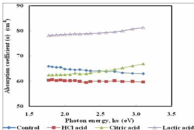
Figure 6 : The absorption coefficient ( $\alpha$ ) of bone/matrices pre- and post-demineralization using different acids as a function of photon energy (hv)
