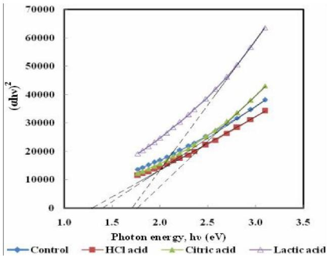
Figure 8 : The variation of  $(\alpha hv)^2$  for bone/matrices pre- and post-demineralization using different acids as a function of photon energy ( $h\nu$ )
