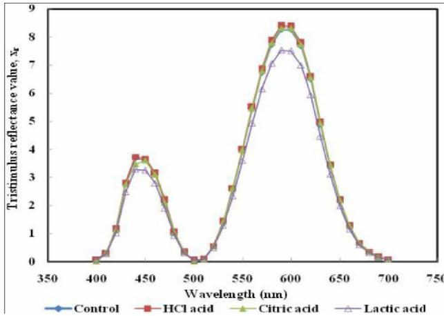
Figure 3 : Variation of the tristimulus reflectance value ( $x_r$ ) with wavelength of bone/matrices pre- and post-demineralization using different acids
