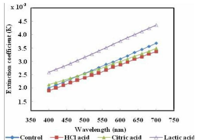
Figure 10 : Variation in the extinction coefficient ( $K$ ) as a function of wavelength ( $\lambda$ ) for bone/matrices pre- and post-demineralization using different acids
