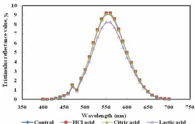
Figure 2 : Variation of the tristimulus reflectance value ( $y_r$ ) with wavelength of bone/matrices pre- and post-demineralization using different acids
