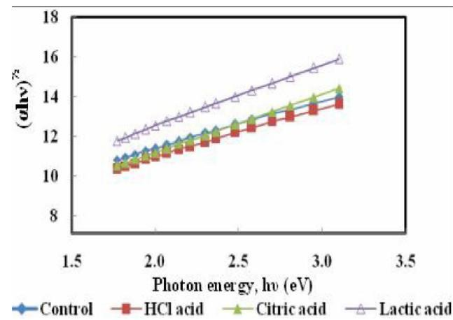
Figure 9 : The variation of  $(\alpha hv)^{1/2}$  for bone/matrices pre- and post-demineralization using different acids as a function of photon energy ( $h\nu$ )
