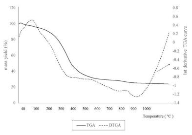
FIG. 4. Thermogravimetric analysis (TGA) of dried food waste.
