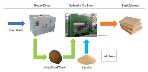
FIG. 1. Proposed concept for particleboard production from mixtures of wood sawdust and dried food waste.
