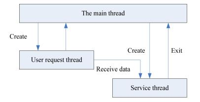
Figure 3 : Management control pattern of emulation management node network
