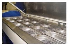
Figure 2 Experimental device for one-side freez-thaw
