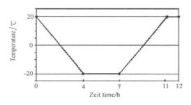
Figure 1 Freezing-thawing cycle of CDF test
