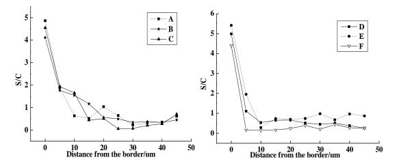
Figure 6 Silica/calcium oxide (S/C) mass ratio in interfacial transition zone
